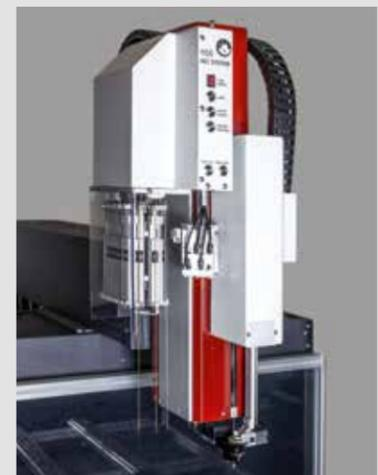
The EDM hole-drilling machine should be set up on a suitable hard industrial floor and preferably on a consolidated concrete floor. Any shielding that may be necessary in conformity with the EMC Directive is not included in the equipment supplied by Mitsubishi Electric. Unloading by forklift truck – no unloading by crane!
