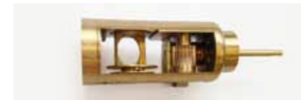
Below Miniature rotating sample stage for operation at a temperature of down to 2 Kelvin (-271°C)
