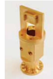
Left Sample stage for measuring physical properties of materials in a vacuum and at low temperatures
