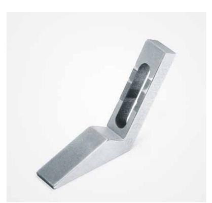
Rake tooth of VA 1.4301, of which the customer ordered several parts. Möderer initially produced a plate, then cut the slot through all the parts and finally wire-cut the exterior contour of all the parts at night during unmanned operation.
