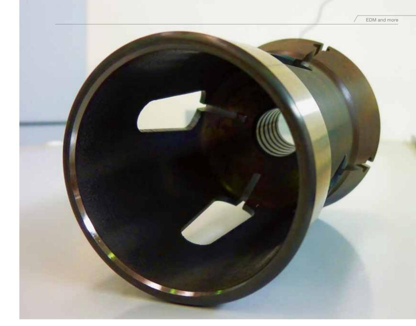
Semi-finished collet with a wire-cut pilot bore and overmeasure for skim cutting. problems. After a certain number of workpieces, rethreading failed to work properly, so the process had to be stopped."
