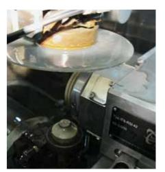
Wire EDM dressing of CBN and diamond grinding wheels with metallic binders:
