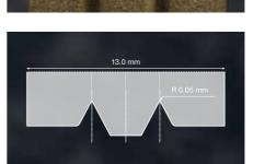
Left Grinding wheel with inner radii of 0.05 mm
