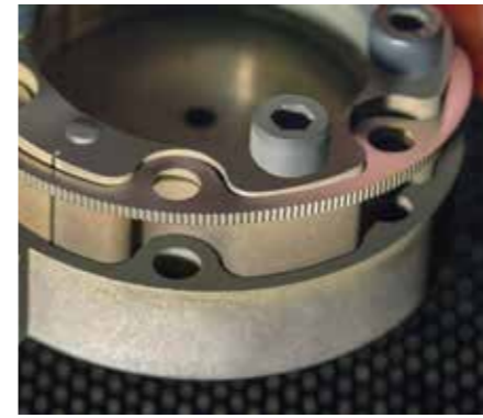
Auxiliary configuration for a 360° cut
