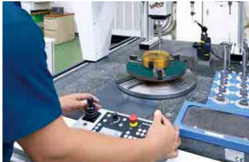
The dies produced with the use of EDM systems are subsequently checked with the coordinate measuring device.
