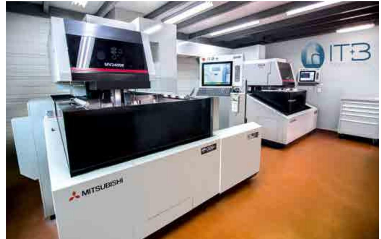
To ensure high precision, ITB Innovation operates its MV1200R and MV2400R wire-cutting machines in an air-conditioned room with a controlled temperature.
