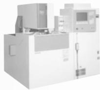
Introduction of the new FX Series with its new revolutionary design principle (fixed table/travelling column principle).
