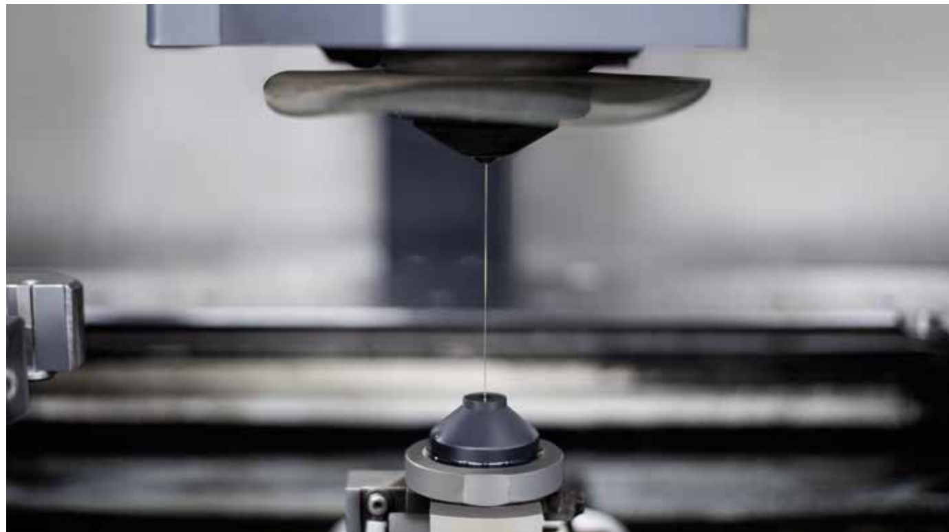
For the machining of precise geometries in hard materials, there's no alternative at Schäfer Feinmechanik in Oberndorf an der Salzach to wire EDM as a cost-effective and high-accuracy production method.
