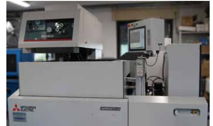
In the Farina Marco workshop, the Mitsubishi Electric MV2400S is used for the production of punches and dies for deburring tools.
