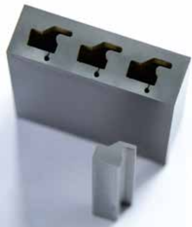
Maximum precision is called for in the machining of replacement parts for punching and cutting tools for the production of tiny components in medical technology and telecommunications.
