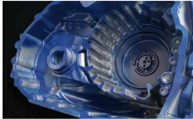
Example of a fairly complex and extensive aluminium part, deburred and cleaned with a tool from the company in Cantù
