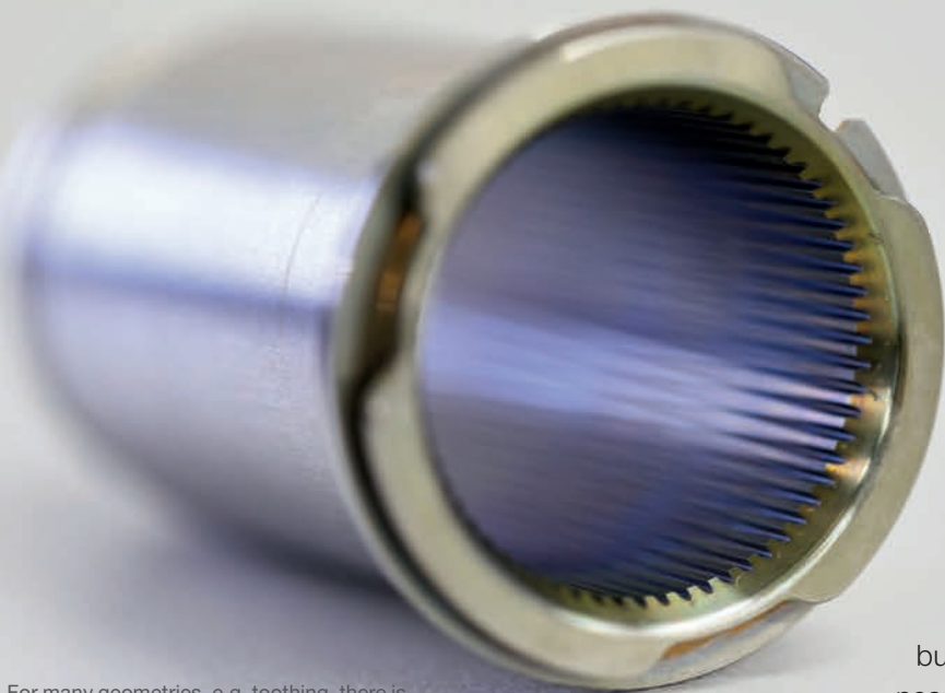
For many geometries, e.g. tothing, there is no alternative to wire-cutting
