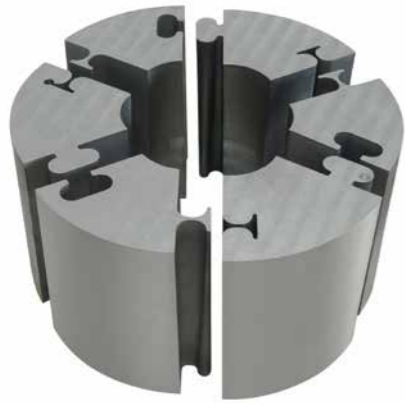
The blank is for an RTM core for the "carbon-fibre aircraft wheel rim" development project, here after 5-axis wire-cutting. The initially closed ring is divided into six segments.
