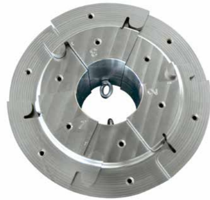
Underside of the core after milling.
