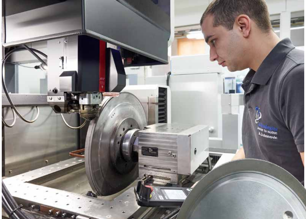
ITS RS180 rotary spindle application: profiling and dressing of metal-bonded diamond and CBN grinding wheels.
