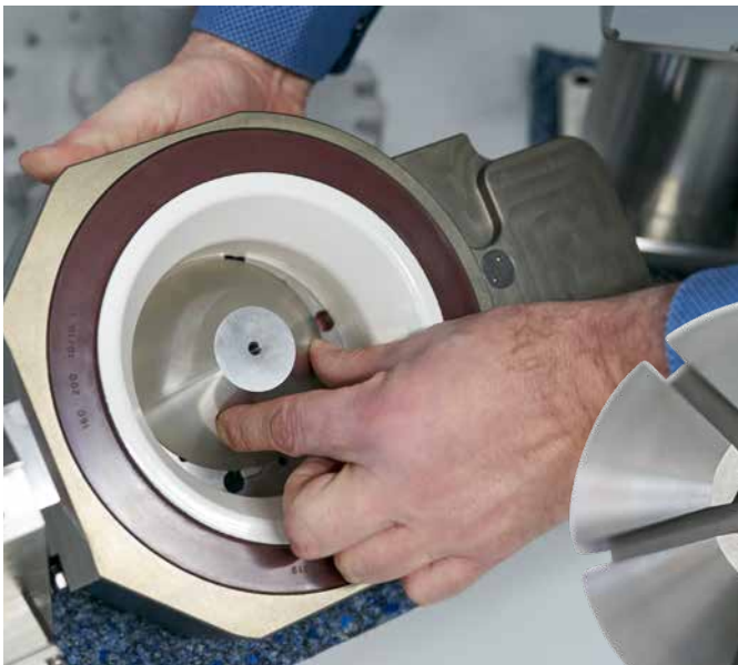
ITS-MA2-i-115 hollow axis application: mandrel groove machining
