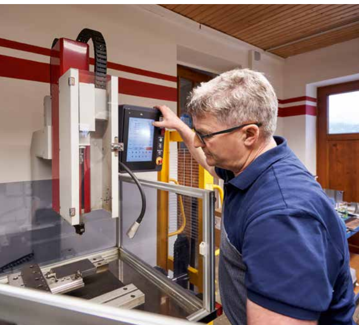
Continuous clamping system – start-hole drilling machine for wire-cutting machine
