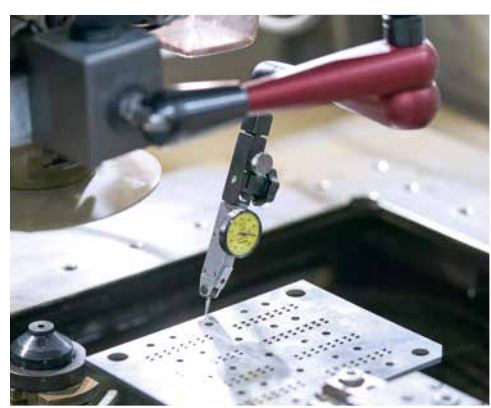
Toolmaker Eduard Steinke aligning the tool
