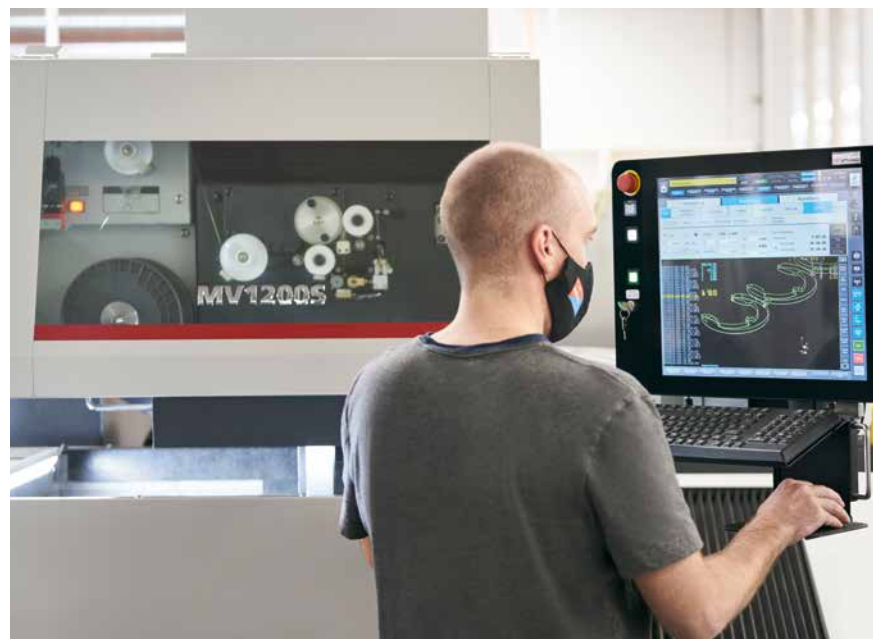
Monitoring the currently running program for the production of special snap rings
