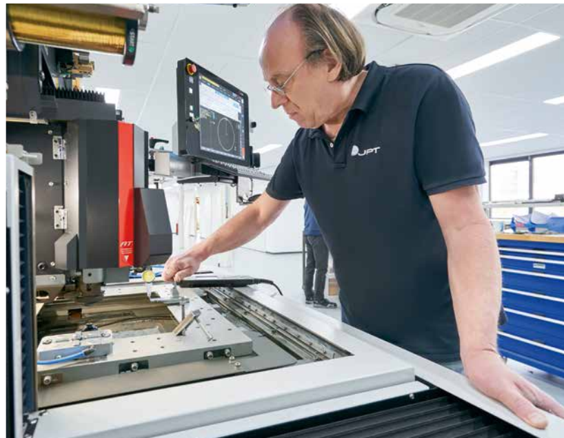
The workspace, fully accessible thanks to the lowerable tank, makes set-up so much easier.
