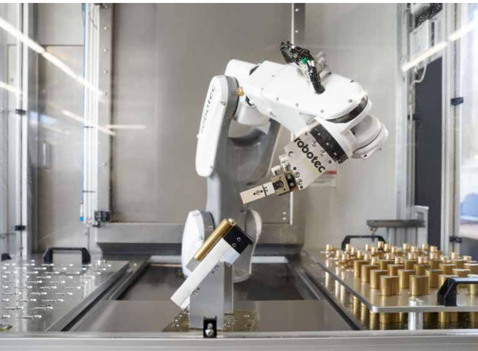
The lock cylinders are fully automatically machined in a robotic cell.
