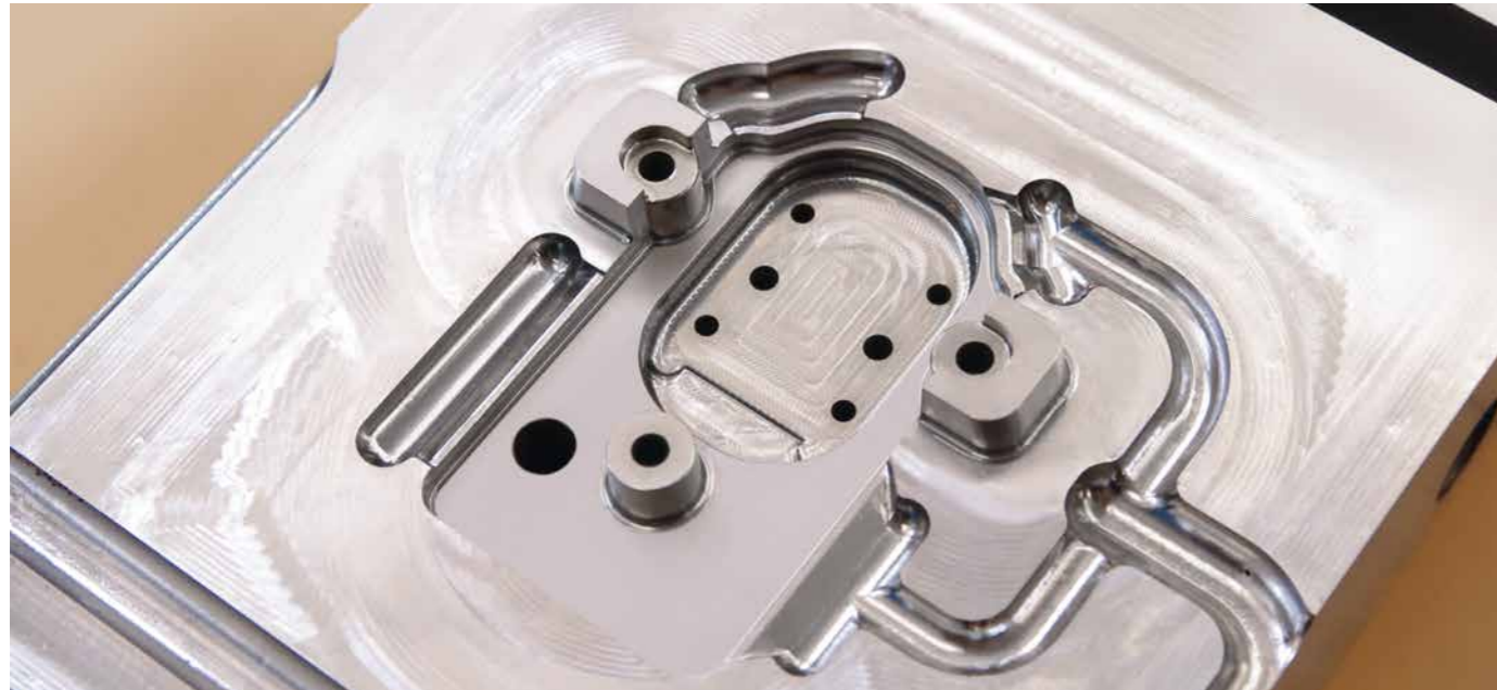
Cut out of hard steel with precision, a variety of openings have to be created in steel die casting and injection moulds for mould inserts, plungers, slides and ejectors.
