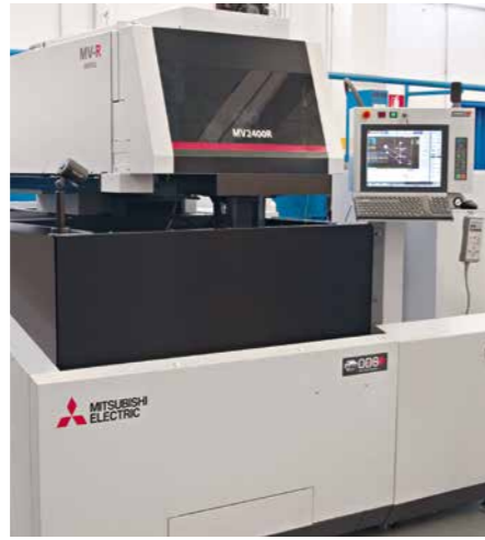
The MV2400R wire EDM machine at DTM in Badalona produces mould inserts with precision and value for money.
