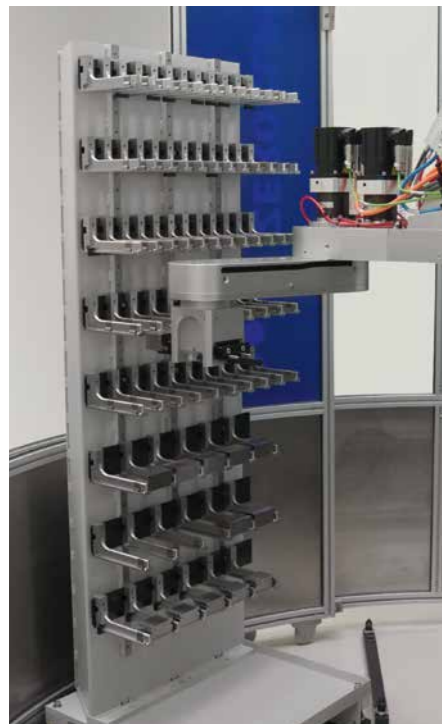
High productivity around the clock: ZeroClamp designs special robots on the Scara principle that load and unload turning and milling centres from individually configured workpiece and tool stores.
