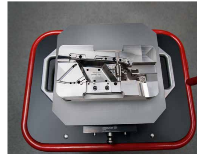
Insert for a 4-cavity mould (recessed grip)
