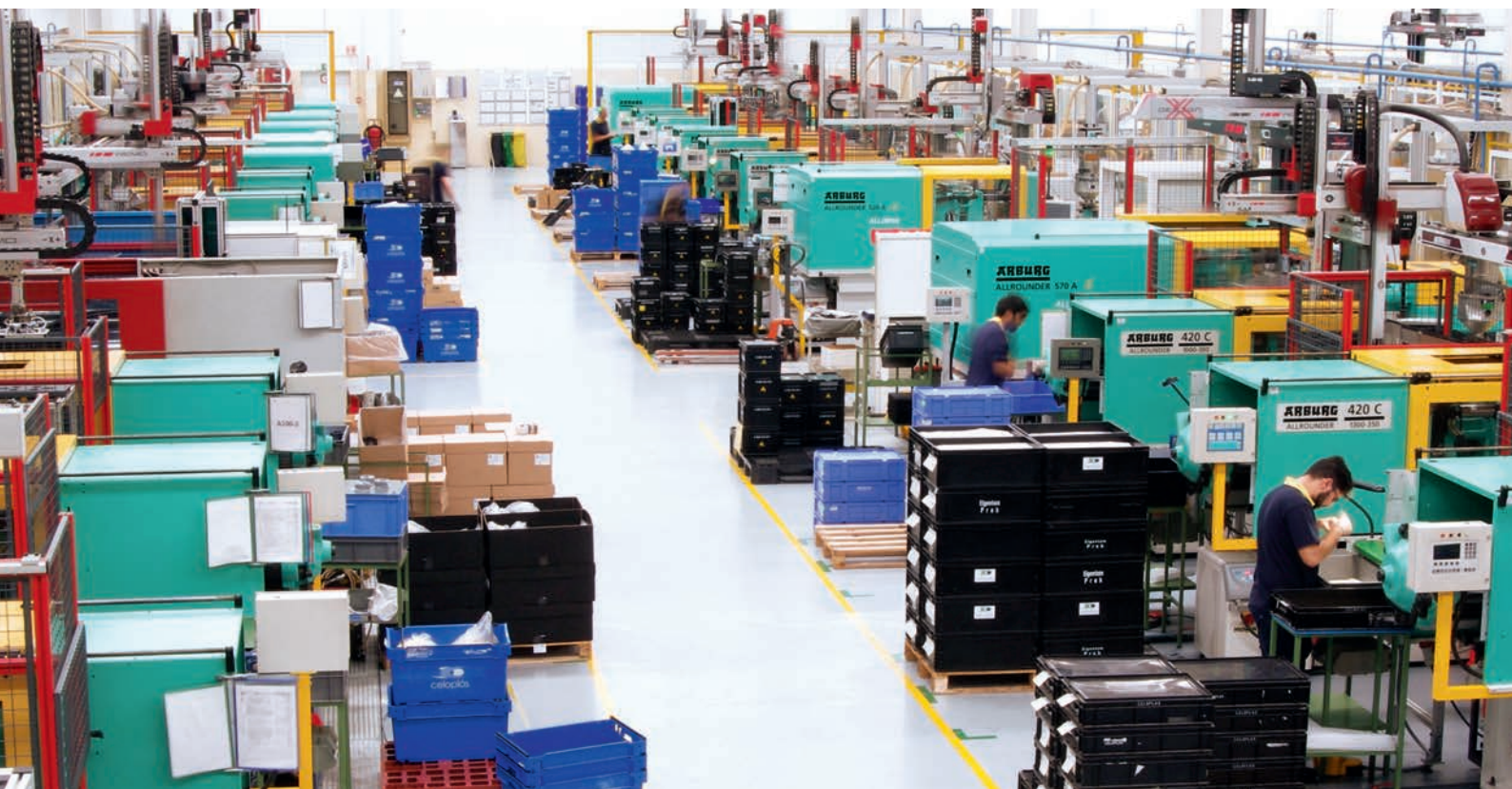
Automated injection moulding of high-grade interior components and plug connectors at Celoplás in Portugal, component supplier to the global vehicle engineering industry.
