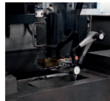
The FA30-S Advance was equipped with an extended Z-axis and a widened work tank so that large sliding mandrels would fit on the machine.
