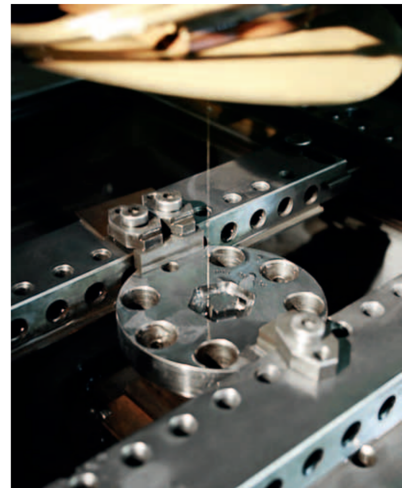
A small tool being machined on the PA20. Here again the workpiece (bottom) is carried by a special holder.
