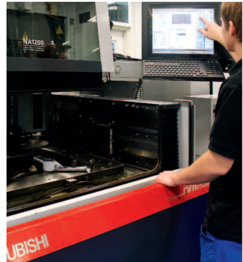
Thanks to its tubular direct drives, the NA1200 Essence is highly precise and is the ideal addition to the WAFIOS machine park.
