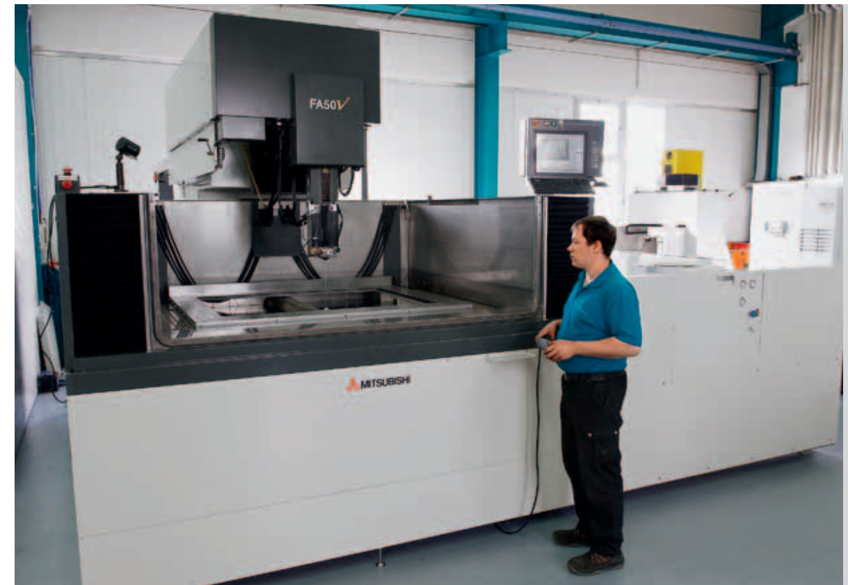
Components measuring 2000 x 1600 x 600 millimetres can be machined on the FA50-S Advance V.
