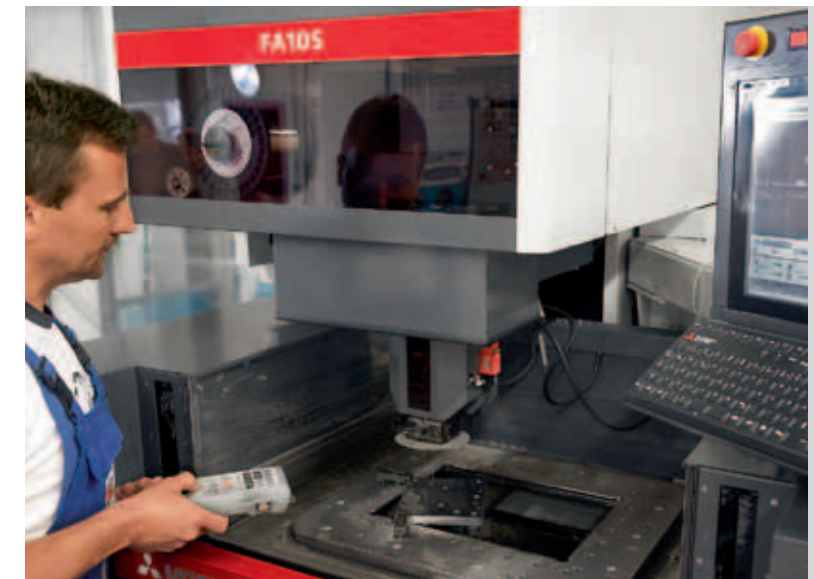
Exact positioning of the wire by remote control.
