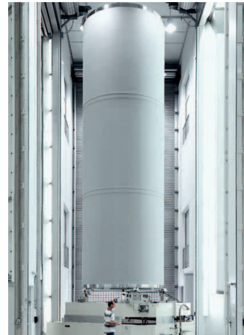
Machining on a grand scale: The boosters of Ariane 5 have a diameter of about 3 m and a total height of 25 m.
