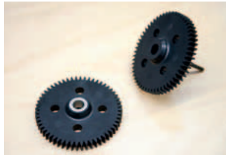
Top The FA10-S Advance cuts tool components of different kinds – in this case a gearwheel mould. The picture shows the finished injection-moulded plastic gearwheel.
