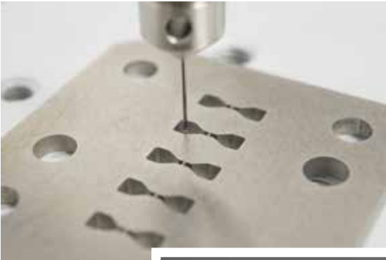
Even the tiniest cavities can be measured thanks to advanced touch probes and CMMs.
