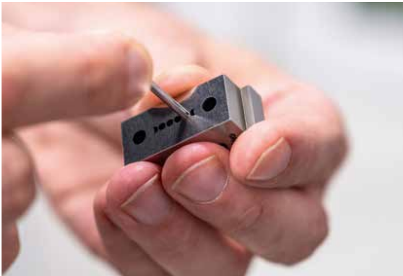
On the wire EDM machines, we use a Japanese approach, with very small tools and a tolerance of 1-2 thousandths striving to achieve the best possible fit.
